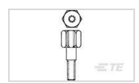
Connector Hardware Accessory Type: Standoff Mounting Stud
