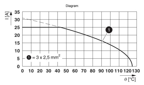
I = current strength,  $\vartheta$  = ambient temperature, 3x 25 A
