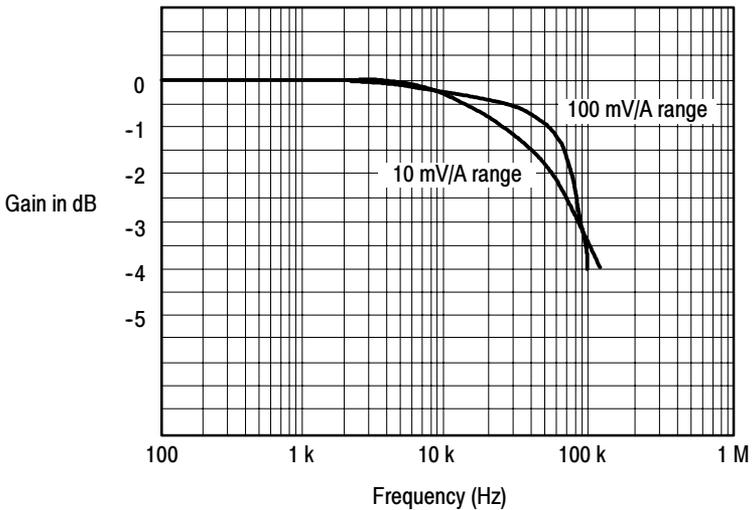
**Figure 6: Gain versus frequency at 1 A peak, typical**
