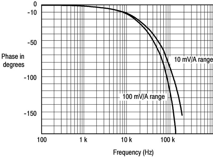
**Figure 9: Phase versus frequency at 1 A peak, typical**
