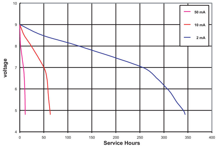
TYPICAL DISCHARGE CHARACTERISTICS AT 21°C (70°F)
