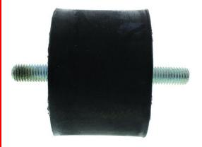
Their elasticity is much greater in all the directions parallel to the armatures than in the perpendicular direction. The rubber works based on compression or shear depending on the direction it is placed in at installation time. This direction is made according to the use and the objective.
