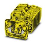
Mini feed-through terminal block, Connection method: Spring-cage connection, Cross section: 0.08 mm² - 4 mm², AWG: 28 - 12, Width: 5.2 mm, Height: 22 mm, Color: black/yellow, Mounting type: Direct mounting with flange
