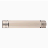
Fuse-link, medium voltage, 31.5 A, AC 22 kV, 51 x 565 mm, full-range, BS, with striker
