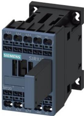
power contactor, AC-3e/AC-3, 9 A, 4 kW / 400 V, 3-pole, 230 V AC, 50/60 Hz, with plugged-on RC element, auxiliary contacts: 1 NO, spring-loaded terminal, size: S00
