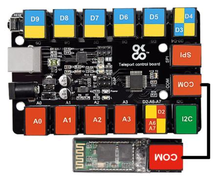
This module is compatible with the TS2178 TelePort control board.
