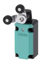
Position switch Metal enclosure 40 mm according to EN 50041 Device connection 1x (M20 x 1.5) 1 NO/1 NC quick action contacts Fork lever operating mechanism with metal lever and plastic rollers 19 mm
