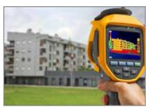
Instruments designed for use in **buildings** are typically used to detect issues within the fabric of construction, and for problems that may be obscured from view or behind walls. Applications include checking the effectiveness of insulation, detecting moisture and leaks, testing underfloor heating systems and central heating
