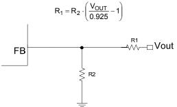
Figure 3. Feedback Divider Network
