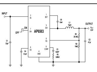
Figure 1 Typical Application Circuit
