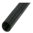
Protective hose, material: PA 6, UV-resistant: yes, flexible, degree of protection: IP68, color: black, flammability rating in acc. with UL 94: HB, inside diameter: 23 mm, Total length: 50 m
