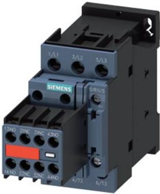
power contactor, AC-3e/AC-3, 32 A, 15 kW / 400 V, 3-pole, 230 V AC, 50/60 Hz, auxiliary contacts: 2 NO + 2 NC, screw terminal, size: S0, captive auxiliary switch, no surge suppressor retrofittable
