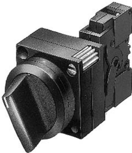
COMMUTATEUR MANETTE, 22MM, ROND, PLASTIQUE, NOIR, MANETTE, COURT, 3 POSITIONS I-O-II, RAPPEL, ANGLE MAN. 2X50 DEG., AVEC SUPPORT, 2 X 1NO+1NF, BORNES A VIS
