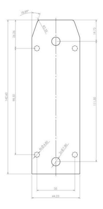
Dashed line shows outline of the mounting boss under PCB board Recommended mounting holes diameter ø3,5mm All dimensions are given within +/-0,5mm tolerance
