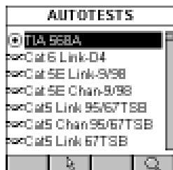
Copper tests are marked with a twisted pair icon.
