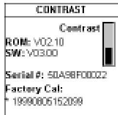
To display the software version #, the hardware version #, the serial #, and the factory calibration data for OMNIScanner, press and hold the Backlight key. The **CONTRAST** screen will be displayed, which contains information that you may need to provide when calling Technical Support.
