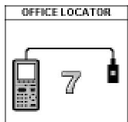
2. Insert the RJ-45 Office Locator adapters into wall outlets in the offices you wish to identify. You can connect any or all of the twelve Office Locators before beginning your test.
