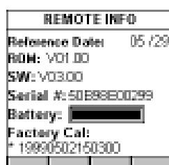
To display software, hardware and serial number information for OMNIRemote, connect the units with the supplied test cable and press the function key.
