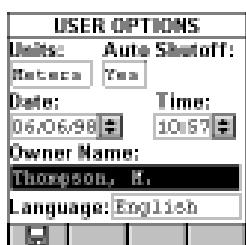
To edit the **Date** use the **→** key to highlight the portions you want to change. Press ENTER to edit the highlighted segment. Use the **↑↓** keys to change the displayed values in increments of 1.
