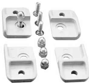
Bracket is molded from fiberglass reinforced polyester. Kit includes four brackets, hardware, and installation instructions. Mounting hole dimensions with mounting brackets installed are  $[G + 2.50(64\text{mm})] \times [H + .50(13\text{mm})]$ .
