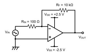
$$V_{OUT} = -\frac{R_F}{R_{IN}} V_{IN}$$
