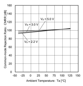
Figure 15. Common-mode Rejection Ratio vs Ambient Temperature
