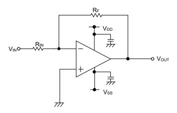
Figure 26. Inverting Amplifier Circuit
