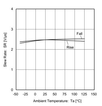
Figure 20. Slew Rate vs Ambient Temperature  $(V_S = 5 V)$
