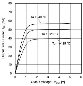
Figure 8. Output Sink Current vs Output Voltage  $(V_S = 5 V)$
