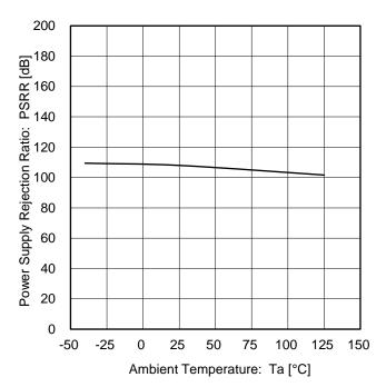
Figure 16. Power Supply Rejection Ratio vs Ambient Temperature
