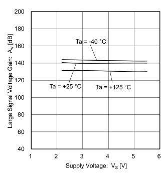
Figure 12. Large Signal Voltage Gain vs Supply Voltage ( $R_L = 10 \text{ k}\Omega$ )
