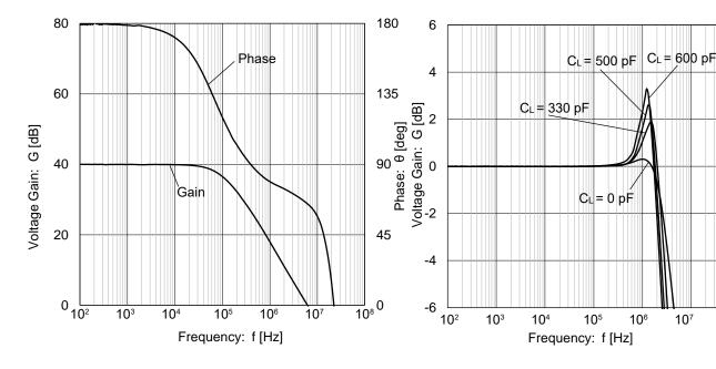
Figure 23. Voltage Gain, Phase vs Frequency  $(V_S = 5 V)$
