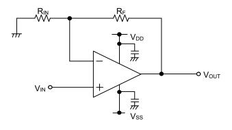
Figure 27. Non-inverting Amplifier Circuit
