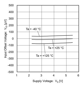
Figure 9. Input Offset Voltage vs Supply Voltage
