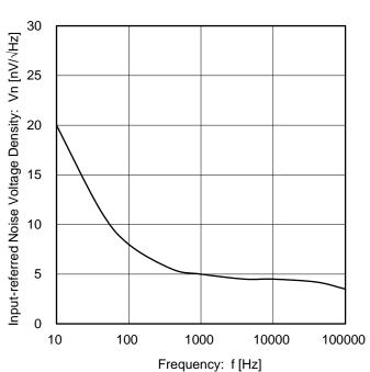
Figure 18. Input-referred Noise Voltage Density vs Frequency (Vs = 5 V)
