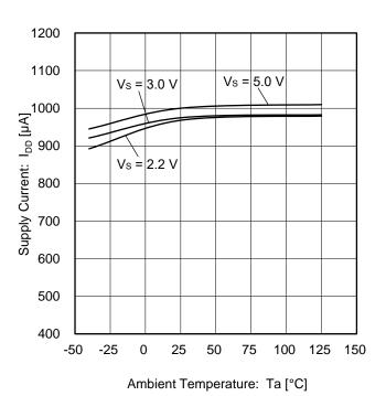
Figure 2. Supply Current vs Ambient Temperature
