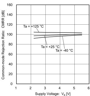
Figure 14. Common-mode Rejection Ratio vs Supply Voltage
