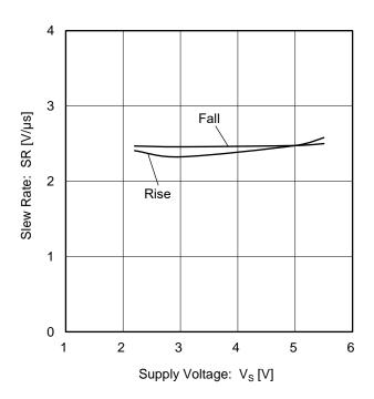
Figure 19. Slew Rate vs Supply Voltage
