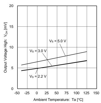
Figure 4. Output Voltage High vs Ambient Temperature (R<sub>L</sub> = 10 kΩ)
