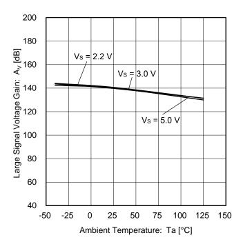
Figure 13. Large Signal Voltage Gain vs Ambient Temperature
