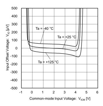
Figure 11. Input Offset Voltage vs Common-mode Input Voltage (Vs = 5 V)
