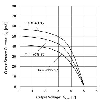
Figure 7. Output Source Current vs Output Voltage  $(V_S = 5 V)$
