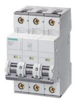
Miniature circuit breaker 400 V D=70 mm 25 kA according to EN 60947-2, 3P, C2
