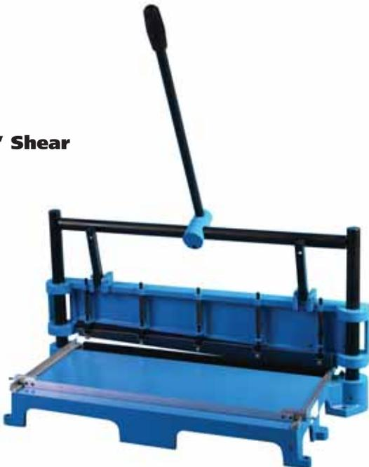
Similar to the above shear but with an increased cutting capacity of 25" (610mm) cutting capacity suitable for cutting printed circuit board laminates, thin metal sheet and aluminium (1.5/2.0mm) or plastic labels / front panel materials. Similar in design and operation to the 18" model except that a fully adjustable front stop and back stop are supplied for batch work.
