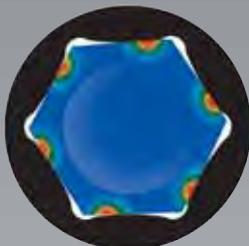
The tolerances on the jaw sizes and square drives of these cold-extruded sockets are as close as if they had been broached. This prevents them slipping off the heads. The consequences: minimum wear on both screws and tools.
