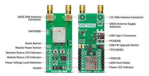
Communication between the SIM7090G and the host MCU is made through a UART interface, using standard UART RX and TX pins and hardware flow control pins (CTS/RTS/RI - Clear to Send/Ready to Send/Ring Indicator) for efficient data transfer. The module defaults to a communication speed of 115200bps, allowing for seamless data exchange over <u>AT commands</u>. Users can change it to the I2C interface supporting up to 400kbps in Fast Mode for the same purpose.
