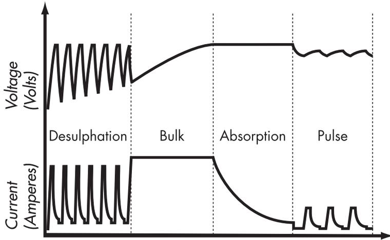
**Desulphation** - Desulphation with pulsing for sulphated batteries.
