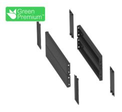
2 side panels for plinth. 400x200mm. Folded sheet steel. RAL 7022. IP 30. IK 10.
