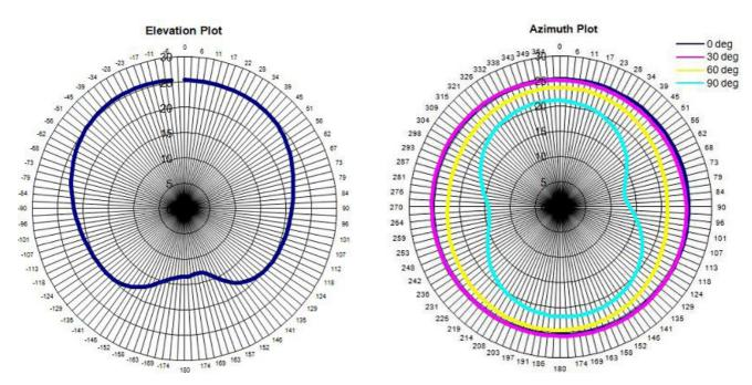
The strength of the PowerHelix antenna technology is its immunity to de-tuning in the presence of dielectric loading, like human tissues. The SL1206 antenna retains efficiency and polarization near the human body. Conventional antennas lose 5-10dB of gain in similar circumstances.
