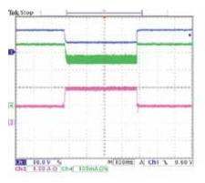
Fig.6 shows the LED current during an input step change from 13.5 to 42V and back to 13.5V (similar to a clamped load dump). It can be seen that the LED current drops briefly when the input voltage jumps, but there are no overshoots.
