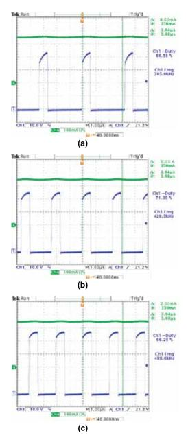
Fig. 5 shows the operation of the converter during cold crank conditions as the input voltage decreases from 13.5V to 6V and increases back to 13.5V. In these cases, the input current reaches the limit set and the output current drops correspondingly. Thus, the LEDs continue to glow, but with reduced intensity. Once the voltage ramps back up, the output current goes back to its normal value and the converter comes out of the input current limit.
