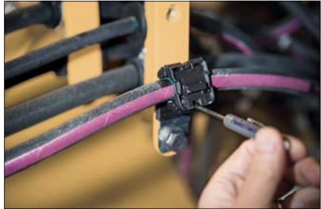
Ratchet P-Clamp - A more versatile way to mount and clamp cables.
