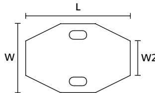
Identification tags with either two, four or six fixing holes.
