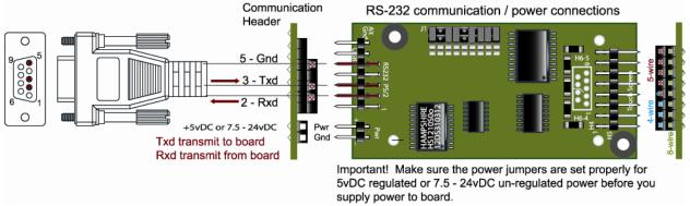
Note: A standard IDC RS-232 (DB-9) to 10-position dual row socket jumper cable assembly may be used. Pin out: 1-1, 2-3, 3-5, 4-7, 5-9, 6-2, 7-4, 8-6, 9-8, NC-10
