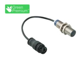
inductive sensor XS6 M18 - L62mm - brass - Sn8mm - 24..240VAC/DC - term. 0.15m
