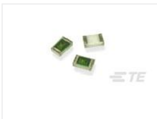
TE Part #1614352-2 RN 0603 20K 0.1% 10PPM CUT LEN
