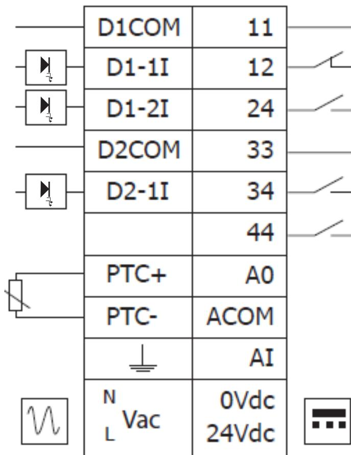
**Note** - 206-073 (430A) to 206-077 (500A) will not have the option of 24VDC. The terminals will be removed.
