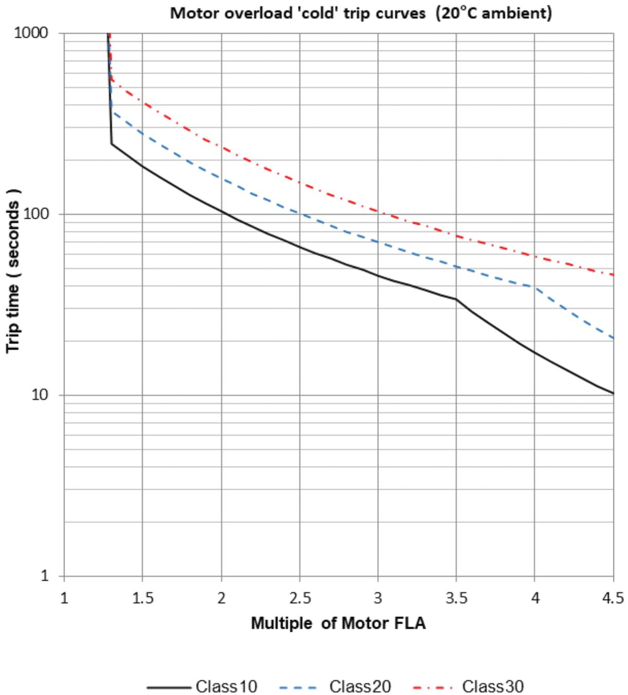
**Note** - When the overload has tripped, there is an enforced cooling time to allow the overload to recover before the next start. The 'warm' trip times are 50% of the 'cold' trip time.
