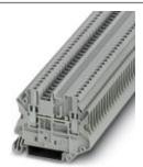
Feed-through terminal block, Connection method: Screw connection, Cross section: 0.14 mm² - 4 mm², AWG: 26 - 12, Width: 5.2 mm, Color: gray, Mounting type: NS 35/7,5, NS 35/15
