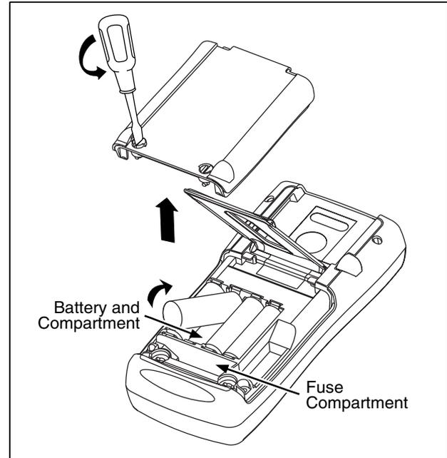
**Figure 4. Replacing the Batteries**
