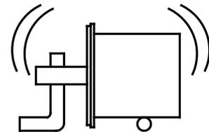
The sensor is non position sensitive offering a similar level of sensitivity whatever its position and has been designed for use with analogue or digital circuitry. The sensor reacts when disturbed by giving a fleeting change of state (ie n/o to n/c or vice versa)
