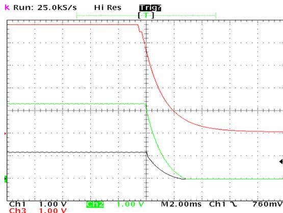
Fig. 11. Scope plot showing the ratiometric power-down sequence of two Austin Lynx™ II series modules. Upper waveform shows the tracking voltage while the two lower waveforms are the output voltages.
