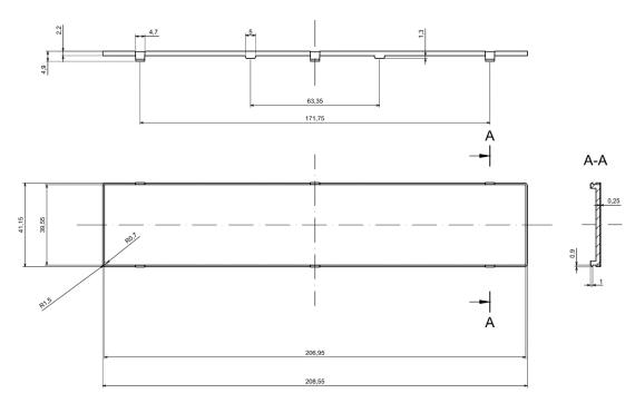
All dimensions are given within +/-0,5mm tolerance
