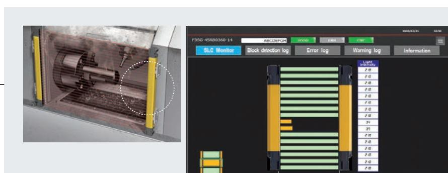
The image shows a machine with a light curtain sensor. Below it is a screenshot of a 'SLC Monitor' software interface. The interface displays a 'Light Intensity' graph with multiple horizontal bars representing different light levels. The graph shows a significant drop in light intensity for one of the bars, indicating a fault. The software also includes tabs for 'Block detection log', 'Error log', 'Warning log', and 'Information'.
