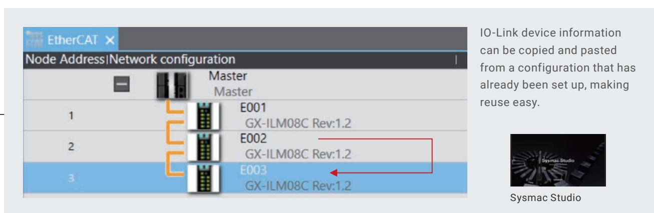
IO-Link device information can be copied and pasted from a configuration that has already been set up, making reuse easy.
