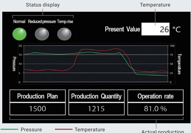
Simultaneously monitoring the pressure and temperature of oil enables pressing conditions to be maintained and controlled. This ensures a consistent finish and raises the standard of pressing quality.
