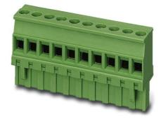
Plug component, nominal current: 12 A, rated voltage: 250 V, pitch: 5.0 mm, no. of positions: 9, type of connection: Screw connection
