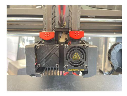
Note: If the Hyper Speed Auto Calibrator is not installed properly, you **cannot** proceed to the next step. Please make sure that the Hyper Speed Auto Calibrator is installed in place.
