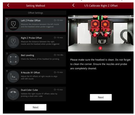
2. Prepare a 0.3mm feeler gauge. Adjust the distance between the nozzle and the build plate according to the prompts on the screen. Make sure the you can feel some resistance as the feeler gauge moves between the nozzle and build plate. Do not press hard on the build plate.
