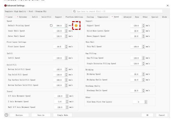
4) In Standard Mode / Hyper Speed Mode, when save the template or slice the model, a warning pop-up window will appear when the speed, acceleration, and Volumatic flow rate exceed the threshold.
