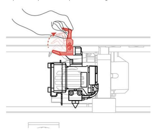
3. Hold the black handle and pull the interchangeable hot end out horizontally.
