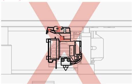
2) If the pin on the red handle is not aligned with the groove on the extruder, you can't close the red handle. Make sure the red handle is fastened.
