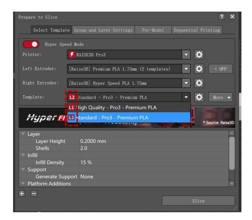
2) ideaMaker will judge all parameters related to speed, acceleration and flow rate in the current template settings. As long as one parameter value reaches L1 or L2, after the template is saved, it will add L1 or L2 labels to the template (In Standard Mode, labels will not be displayed).
