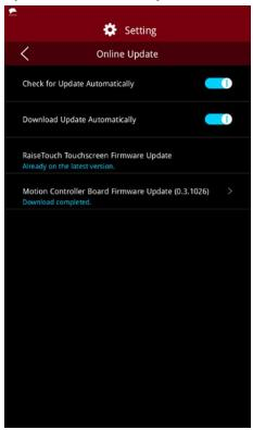
2. The printer will automatically detect the RaiseTouch Hyper Speed firmware and download it. When you see "RaiseTouch Touchscreen Firmware Update" displays: "There is a new firmware version", click it, the printer will automatically download and run the update program.
