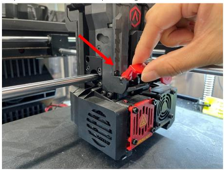
4. Press down the red handle to secure the hot end in place.
