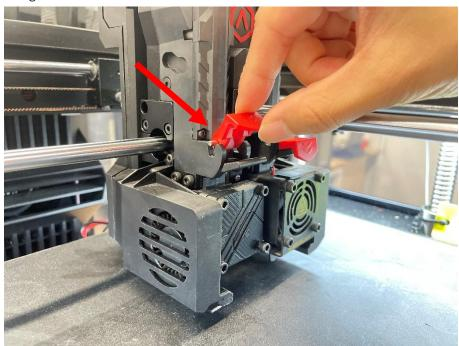
7. Press down the red handle to secure it in place.
