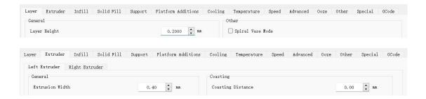
6. After adjusting the parameters, click "Slice" to slice the model.
