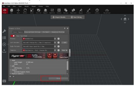
7. After slicing, save the file locally and import it to the printer; or you can directly upload it to the Pro3 series printer to start your hyper speed printing.
