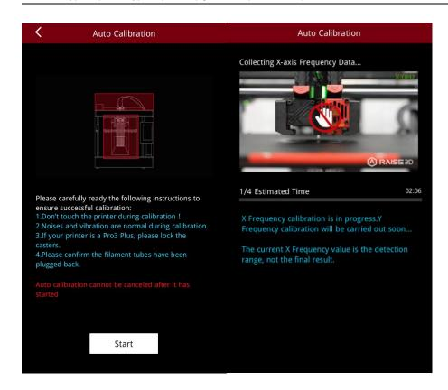
3. After the calibration is finished, the wizard will prompt "Calibration succeeded!". The frequency of the current X/Y axis will be displayed. Click "Confirm" to apply the value and move to the next step.
