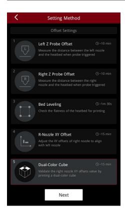
2. After printing, please compare the printed dual-color cube with the sample graphic on the screen, and check whether there is an obvious gap between the color blocks.
