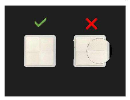
4. If there is a gap between the color blocks, please click "**Retry**" and re-run the 4th and 5th steps of the 5-step Offset Calibration to recalibrate the XY offset value of the right nozzle.
