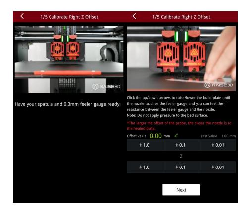
3. After adjusting the distance between the nozzle and the build plate, follow the prompt on the screen to load Hyper Speed PLA filament.
