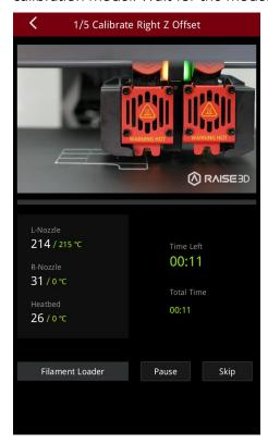
5. After the model is printed, compare the model with the on-screen example. Select the first block that doesn't leak light. The printer will automatically adjust the offset value of the left nozzle.
