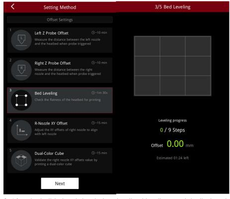
2. After the build plate is leveled, a visualized leveling result is displayed.
