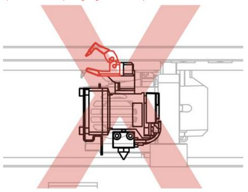
2) When removing, do not pull the hot end upwards.
