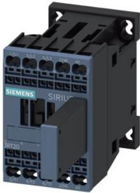
power contactor, AC-3e/AC-3, 12 A, 5.5 kW / 400 V, 3-pole, 230 V AC, 50/60 Hz, with plugged-on RC element, auxiliary contacts: 1 NC, spring-loaded terminal, size: S00
