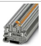
Knife disconnect terminal block, With test socket screws for insertion of test plugs, Connection method: Screw connection, Cross section: 0.14 mm² - 6 mm², AWG: 26 - 10, Width: 6.2 mm, Color: gray, Mounting type: NS 35/7,5, NS 35/15
