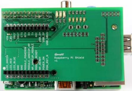
The ShieldRv1.0 is a shield or connecting board that connects the CELLv1.0 to the Raspberry Pi without any additional wiring. It also provides LEDs for the CELLv1.0 status lines.
