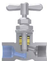
Valve closed position
