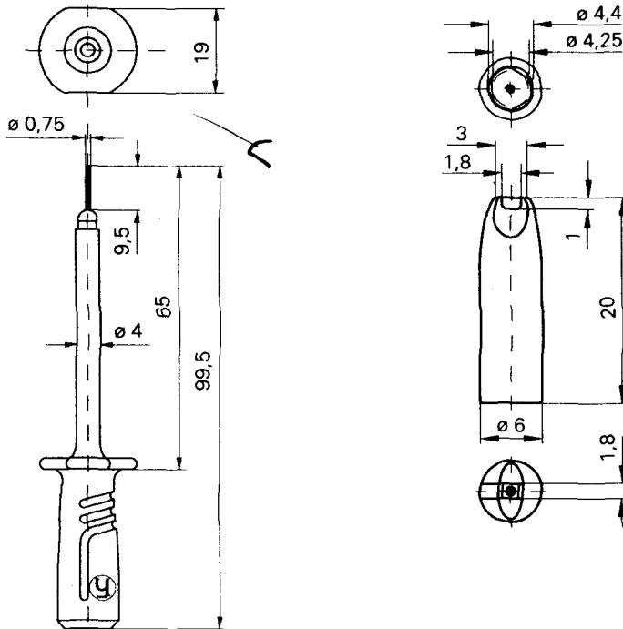
Test probe with elastic shatter-proof insulated sleeve and slim, **spring-mounted** stainless steel tip, 0.75 mm in diameter. This ensures **constant contact pressure without slipping off**, even on the smallest measuring points. Spring-mounted 4 mm dia. connectors and measuring leads can be plugged into the **4 mm dia. socket connection**. Contact safety up to 1000 V is guaranteed when using shock-proof measuring leads (MLB ...) (refer to the range of safety equipment up to 1000 V).
