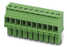
Plug component, nominal current: 8 A, rated voltage: 160 V, pitch: 3.81 mm, no. of positions: 8, type of connection: Screw connection
