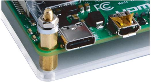
5. Fixed Acrylic protection holder to Raspberry Pi with M2.5 screws.
