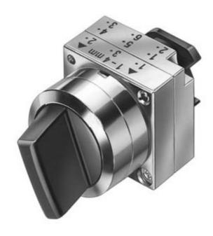
22MM METAL ROUND ACTUATOR: SELECTOR SWITCH MOMENTARY CONTACT TYPE 3 SWITCH POSITIONS I-O -II ILLUMINATED WITH HOLDER CLEAR, SOLVENT-RESISTANT NOT INSCRIBABLE WITH LASER
