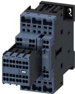
power contactor, AC-3e/AC-3, 25 A, 11 kW / 400 V, 3-pole, 24 V AC, 50 Hz, auxiliary contacts: 2 NO + 2 NC, spring-loaded terminal, size: S0, removable auxiliary switch
