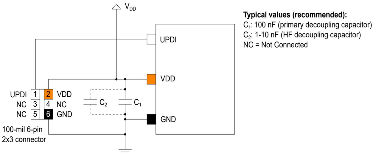
The decoupling capacitor between VDD and GND must be placed as close to the pin pair as possible. Include the decoupling capacitor even if the UPDI connector is not included in the circuit.
