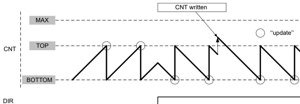
The counter value in the Counter (TCEn.CNT) register can be changed while the counter is running. The write access to the TCEn.CNT register has higher priority than count, clear or reload and will be immediate. The direction of the counter can also be changed during normal operation by writing to the Direction (DIR) bit in the Control E (TCEn.CTRLE) register.
