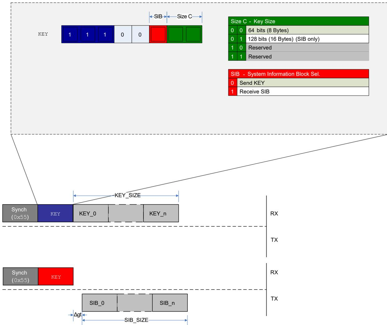
Figure 34-17 shows the transmission of a key and the reception of a SIB. In both cases, the Size C (`SIZE_C`) field in the operand determines the number of frames being sent or received. There is no response after sending a `KEY` to the UPDI. When requesting the SIB, data will be transmitted from the UPDI according to the current guard time setting.
