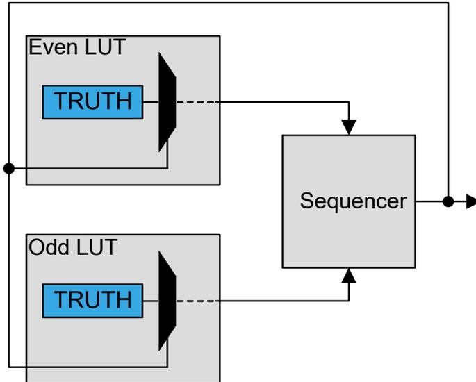
When selected ( $INSELy = FEEDBACK$  in  $LUTnCTRLx$ ), the sequencer (SEQ) output is used as input for the corresponding LUTs.
