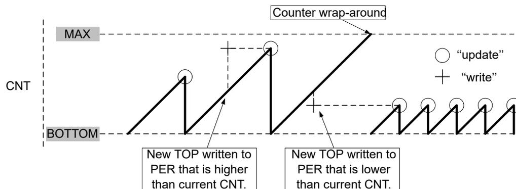
A counter wraparound can occur in any mode of operation when up-counting without buffering. This happens because the TCEn.CNT and TCEn.PER registers are continuously compared. If a new TOP value is written to TCEn.PER that is lower than current TCEn.CNT, the counter will wrap first before a compare match happens.
