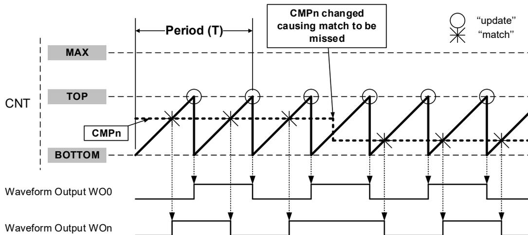
The figure below shows how the waveform can be inverted by changing the CMPn during run-time.
