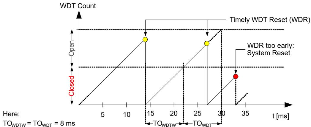
The Window mode is enabled by writing a non-zero value to the WINDOW bit field in the Control A (WDT.CTRLA) register and disabled by writing it to  $0 \times 0$ .
