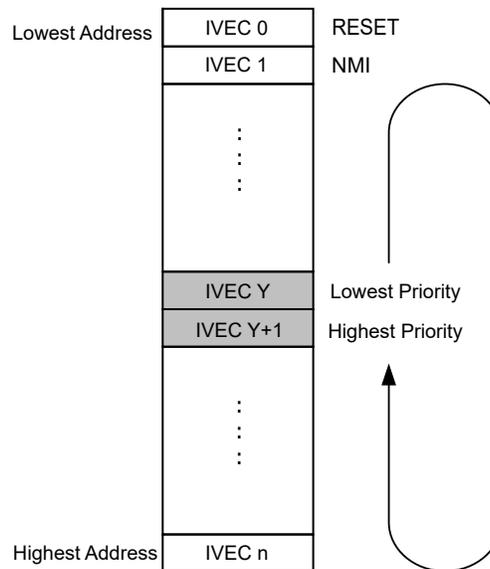
Here, value Y has been written to CPUINT.LVL0PRI so that the interrupt vector Y+1 has the highest priority. Note that, in this case, the priorities will wrap so that the lowest address no longer has the highest priority, not including RESET and NMI, which will always have the highest priority.
