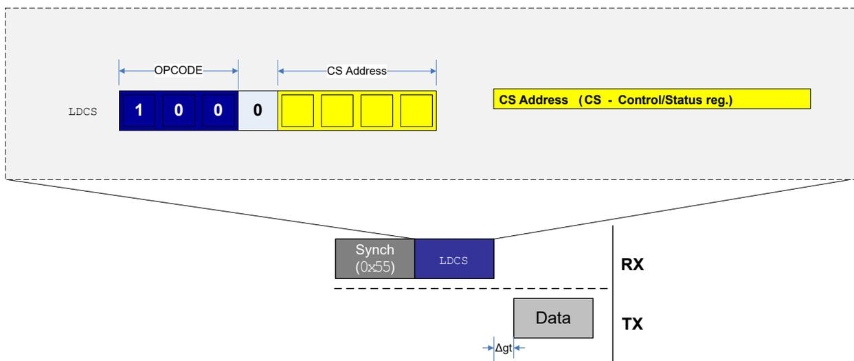
Figure 34-13 shows a typical example of `LDCS` data transmission. A data byte from the `LDCS` is transmitted from the UPDI after the guard time is completed.
