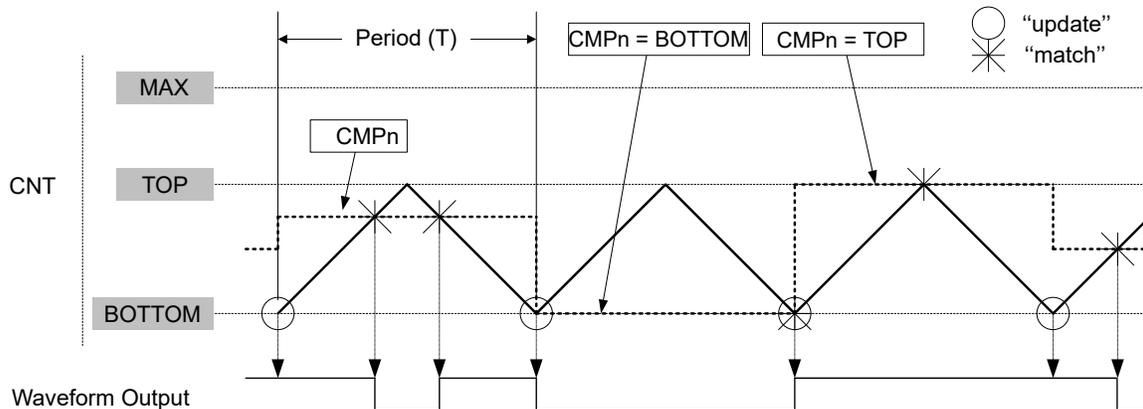
The Period (TCEn.PER) register defines the PWM resolution. The minimum resolution is two bits (TCEn.PER = 0x0003), and the maximum is 16 bits (TCEn.PER = MAX).
