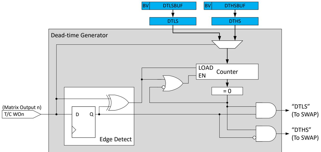
Figure 24-5 shows the 8-bit dead-time counter is decremented by one for each peripheral clock cycle until it reaches zero. A nonzero counter value will force the low and high side outputs into their OFF state.
