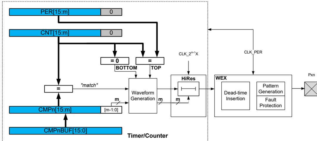
When the high-resolution extension is enabled, the timer/counter must run from a non-prescaled peripheral clock.
