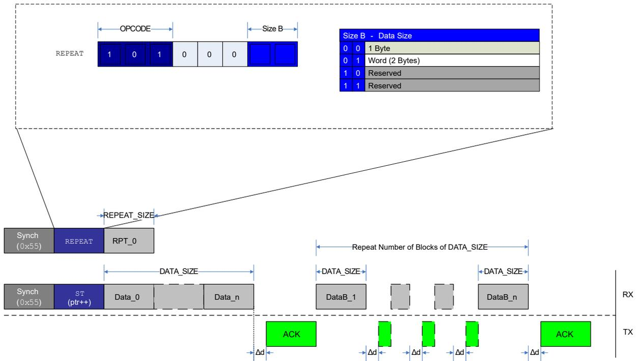
Figure 34-15 gives an example of a repeat operation with an ST instruction using pointer post-increment operation. After the REPEAT instruction is sent with RPT\_0 = n, the first ST instruction is issued with SYNCH and instruction frame. The next n ST instructions are executed by only sending data bytes according to the ST operand DATA\_SIZE and maintaining the Acknowledge (ACK) handshake protocol.
