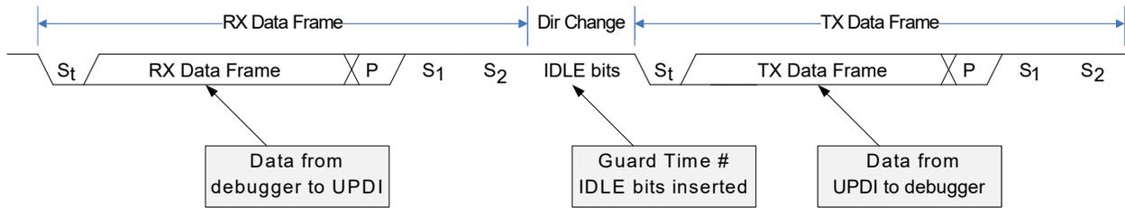
The UPDI guard time is the minimum Idle time that the connected debugger will experience when waiting for data from the UPDI. The maximum Idle time is the same as time-out. When the synchronization time plus the data bus accessing time is longer than the guard time, the Idle time before a transmission will be more than the expected guard time.
