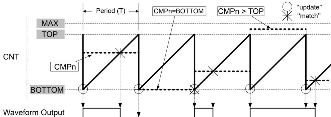
The TCEn.PER register defines the PWM resolution. The minimum resolution is two bits (TCEn.PER = 0x0002), and the maximum is 16 bits (TCEn.PER = MAX-1).
