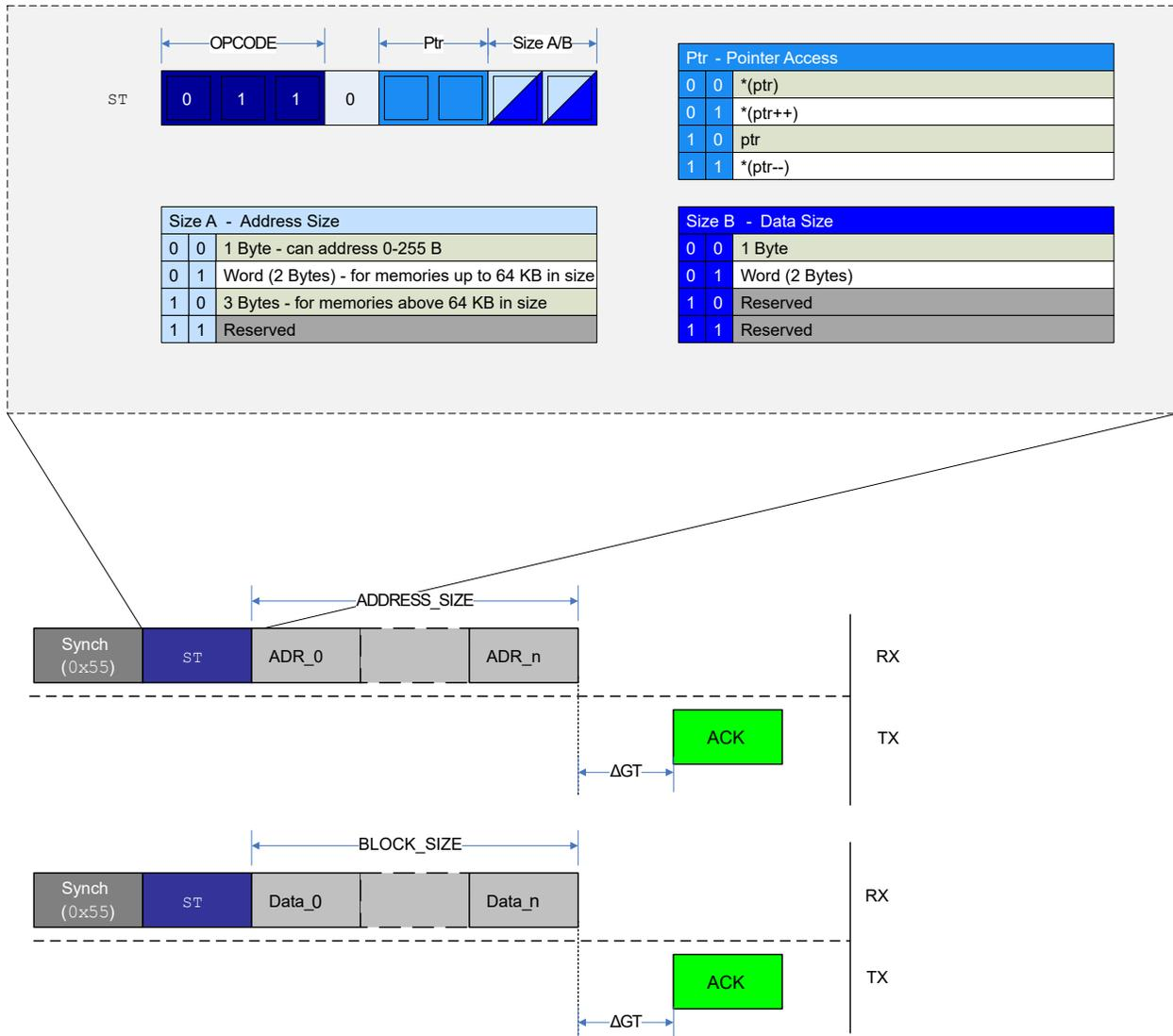
Figure 34-12 gives an example of an `ST` instruction to the UPDI Pointer register and the storage of regular data. A SYNCH character is sent before each instruction. In both cases, an Acknowledge (ACK) is sent back by the UPDI if the `ST` instruction was successful.
